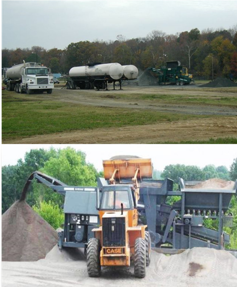
Figure 3: Stockpile and screening aggregate
