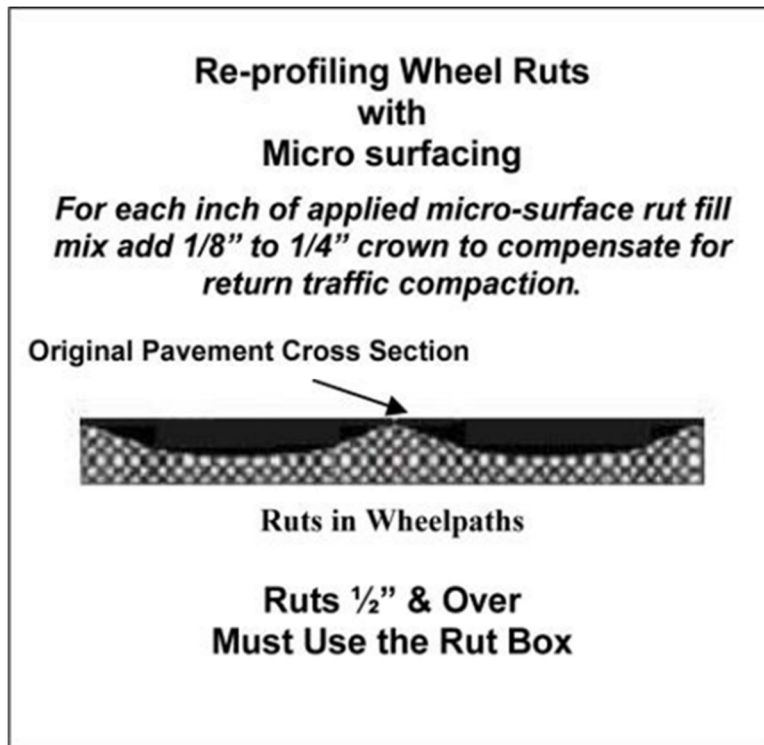
Figure 15: Wheelpatch re-profiling illustration
